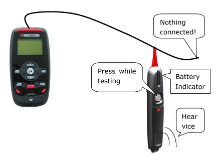
**Battery Low:** When pressing the test button of tone tracer, the battery indicator turn on all the time means battery should be replaced as soon as possible.
