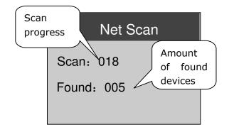
The tester stops scan when it gets to the end of the IP range. User can press [OK] to interrupt a scan progress. Press  $[\uparrow]or[\downarrow]$  to see the device's IP and MAC.
