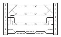
Wires 1-3 are twisted together ,wires 2-6 are twisted together, LCD displays is shown below:
