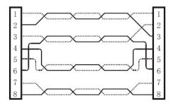
Wire 2 is connected to wire 3 on the other end. See the displays below:
