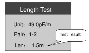
Press[ $\uparrow$ ] or [ $\downarrow$ ] to adjust the capacitance per unit length, and the tester will display as follows:
