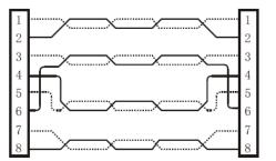
One-end Test pass cable ,tester displays as follow:
