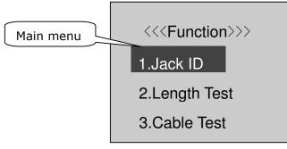
Press [  $\uparrow$  ] or [  $\downarrow$  ]key to select a function in the main menu, and press [OK] key to start the selected function. Press [ESC] key can return to main menu in any function.
