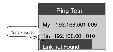
address  $\,$  of the tester must be set first. If these two address are not in the same LAN , the gateway and subnet mask should be set, too.
