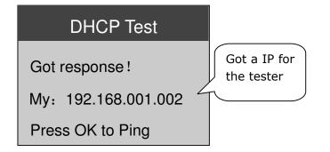
Press [OK] once to ping the DNS server; Press [OK]twice to ping the Gateway; Press[OK] thrice to ping a target IP. Press [SETUP] to set the target IP.
