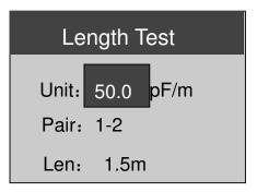
For cables of unknown capacitance per unit length, a cable of known length of the same kind will be as the cable whose length is to be measured is connected to the tester. To reduce the error at maximum, it is suggested to use the cable above 20 meters.
