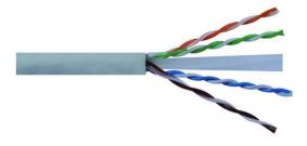
Wave Cables Cat. 6 U/UTP cables are designed to meet the most advanced U/UTP cable applications. Tested to 250MHz, the performance of this cable meets the requirements for PS-NEXT, attenuation, return loss, attenuation-to-crosstalk ratio (ACR) and impedance, making it ideal for high-end transmission links supporting todays networking protocols.
