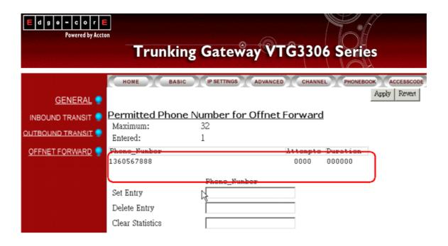
Attention: The telephone number defined in the field of "Offnet To" is the number actually dialed from the remote transfer gateway. In this example, the call is forwarded to offnet mobile phone of China, therefore no area code is required when call is transferred from the gateway in Shanghai.
