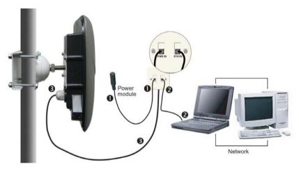
Figure 3-6 Typical TOTAL radio system
